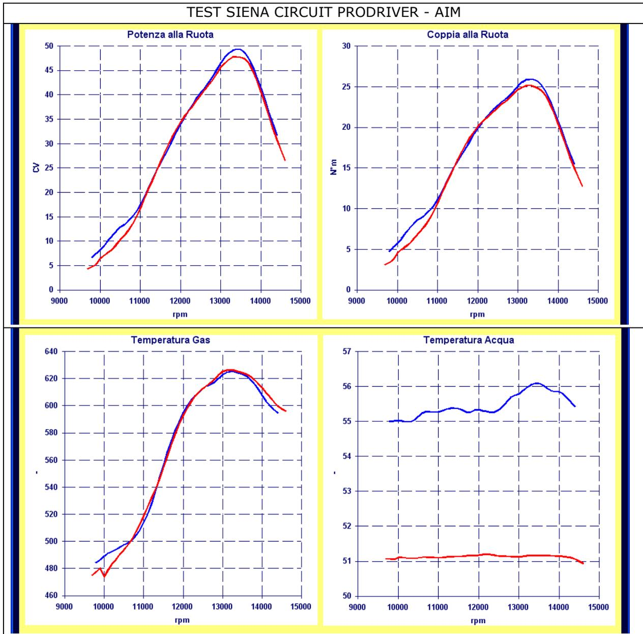
Also in this case we can see that between two runs with the same set-up engine the result, is very similar, here the performance variation is only due to the fact that in a run, the engine had not yet reached the optimum operating temperature.
