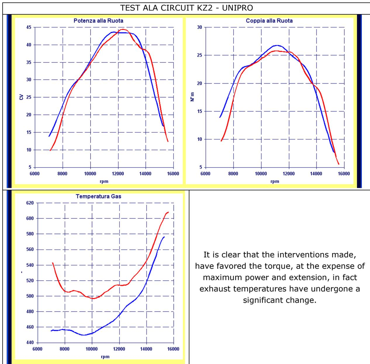
As you can see, thanks to Virtual Dyno each test that you do on the engine, both with technical modifications, or both with operations of jetting and ignition set-up, can be evaluated clearly. So you'll enable to make the optimal choices and therefore may concentrate without doubts about the other steps of fine tuning of chassis and tire.
