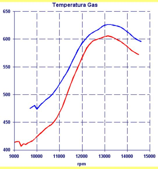
It is clear that the interventions made have allowed to increase the maximum power, and this is consistent with what was happening to the temperature of the exhaust gases, a testimony to the good work of the system and the software Virtual Dyno.
