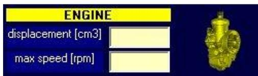
Use of the software is extremely simple, in fact you'll just have to enter the engine displacement and the maximum engine speed, so the software can evaluate the fluid-dynamics conditions in which works the circuit of the maximum of the carburetor.
