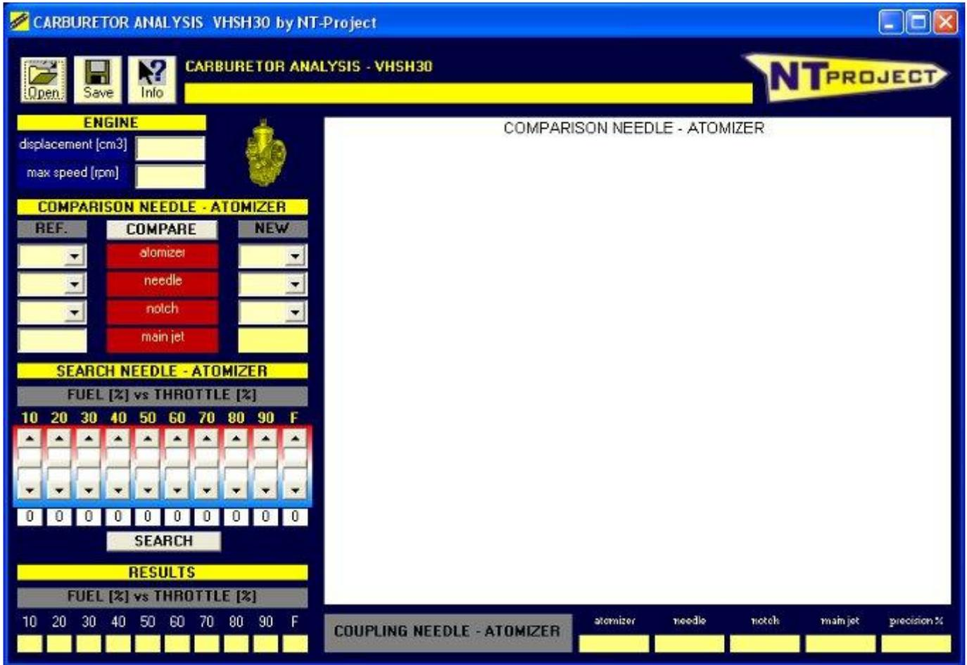
The software **CARBURETOR ANALYSIS** allows to analyze and to find the optimal needle and atomizer for the needs of the engine, the driver, and the track.
