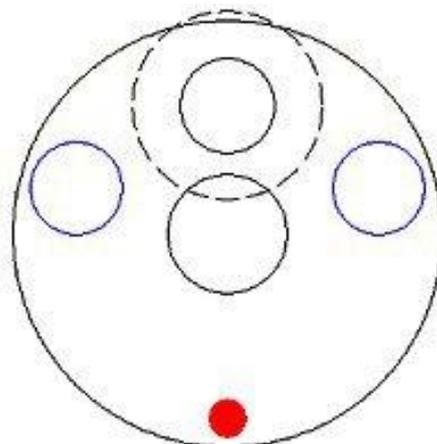
For all these types the software automatically calculates the position and the size of all the counterweights, hollows or holes which must be drilled to obtain the desired result, and shows also the relative drawing. Therefore create a crankshaft with a specific balancing or with a certain inertia will become extremely fast and effective.
