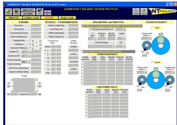
The area of analysis allows to have immediately a complete picture of the status of the crankshaft analyzing **WEIGHT - BALANCING - SYMMETRY and INERTIA**
