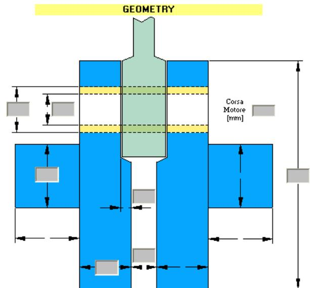
Moreover you can easily indicate the position and the characteristics of eventual holes and counterweights present on the crankshaft.
