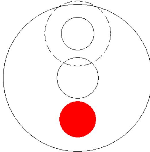
Besides to the numbers, a graphical view of the data entered it is fundamental both to see if the geometry data that have been entered are correct and no mistakes were made, and to evaluate the possibilities of space for any changes that you intend to do. For this reason, the software draws the crankshaft and also creates its image that can be printed.
