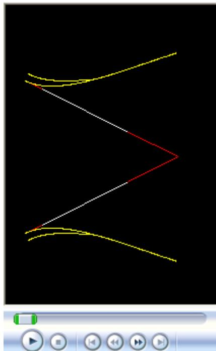
The first result shown by the software REED DESIGN is the behavior of the reed petals choices under varying pressure conditions. The software can handle both the pressure range over which simulate the behavior of both the steps of analysis and the frequency of display..
