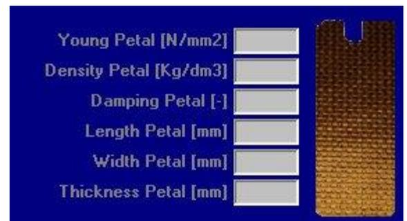
To analyze the displacement of the petal and the associated transition areas are sufficient the size and Young's modulus, while for the dynamic analysis you will also include the density and the damping coefficient, if you know it.
