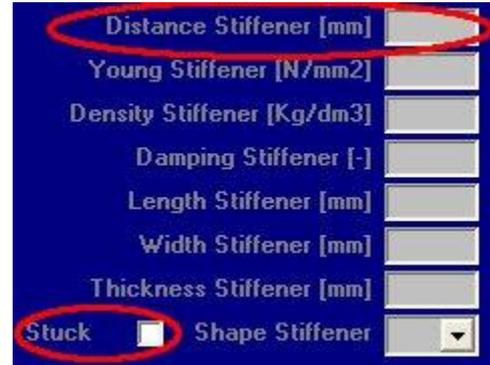
The software REED DESIGN allows to evaluate the behavior also in the case if there is a spacer between the main petal and the stiffener so you can obtain a variable stiffness to vary the pressure conditions.
