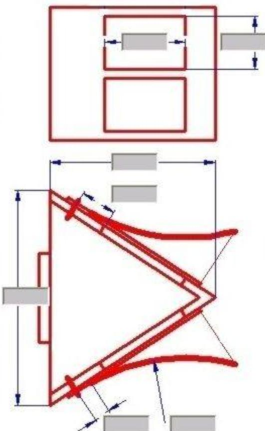
The software REED DESIGN for first requires the data entry of the reed valve for which you want to identify the most suitable reed petals. These are the dimensions that characterize the shape and those of the ports where the flow passes.
