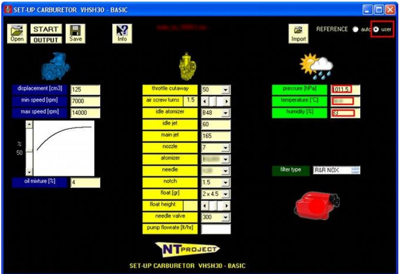
When doing the calculation the software SET-UP Carburetor will show you the graphs putting your carburetion of reference (blue line) and the new (red line) due to changes you have made (for example, new weather conditions)
