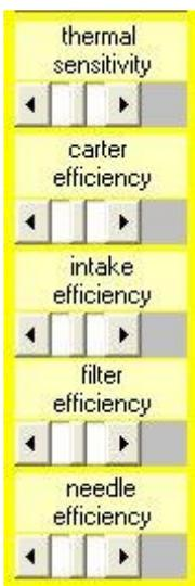
Besides the changes to the engine, or the change of engine model, it can happen that are made different heat treatments at cylinder that alter the heat transfer and therefore make the engine more or less sensitive to atmospheric conditions, in the software SET-UP Carburetor you can handle this too, allowing you to always have the software configured for your situation.
