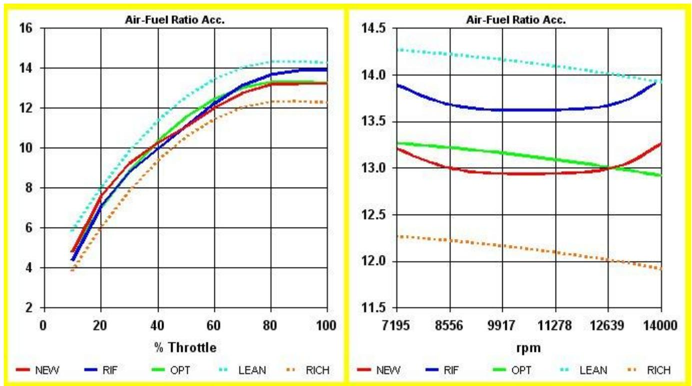
In the graphs you can see how was the carburetion with the jetting initially inserted (blue line) and that due to the jetting modified (red line), which must be as close as possible to that of the optimum carburetion.
