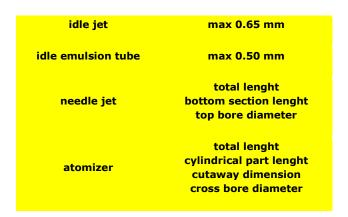
Therefore working on the calibration elements in compliance to the permitted tolerances, thanks to the software is possible to find the solutions that allow to improve the basic jetting, with an elasticity significantly higher compared to that which can be obtained by acting simply on the air screw, the needle notch and the main jet.
