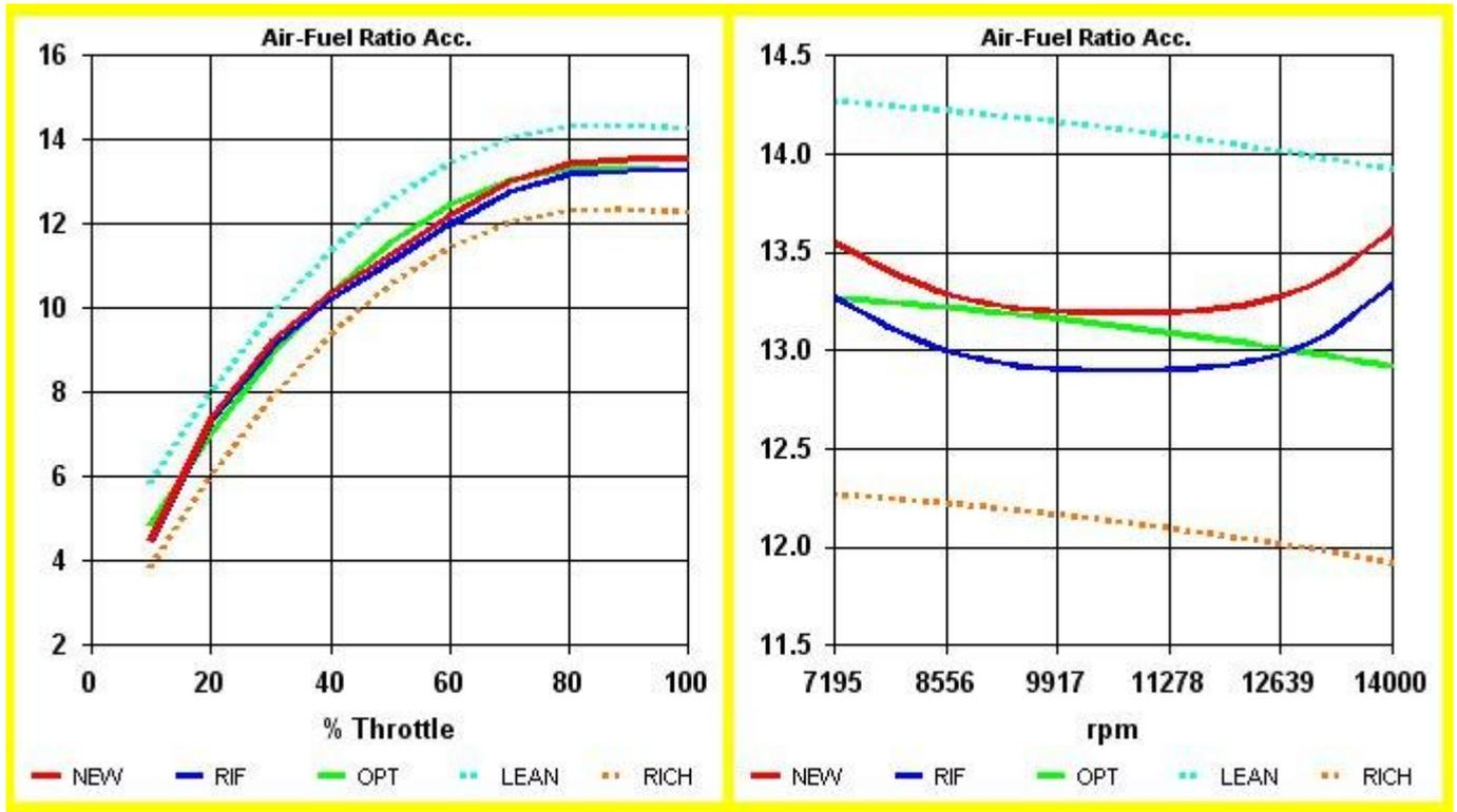
Moreover, the software SET-UP Carburetor will give the indications on how to change the jetting to return to your carburetion you have taken as a reference.
