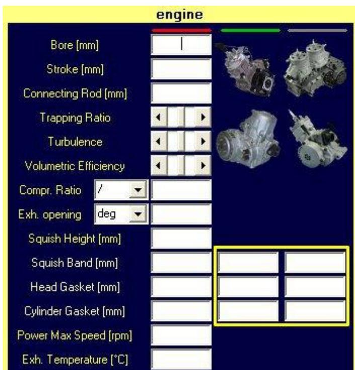
Among the parameters on which it intervenes in the fine tuning there are certainly the squish, the compression ratio and the opening angle of the exhaust ports, and these are changed by adjusting the thickness of the cylinder and head gaskets, for this in the software over the standard configuration, you can enter other combinations of these parameters (yellow rectangle).
