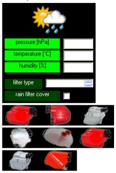
Then you will have to enter the current carburettor setting, the atmospheric conditions for which you want to optimize the carburetion, and the type of the filter used on the engine.
