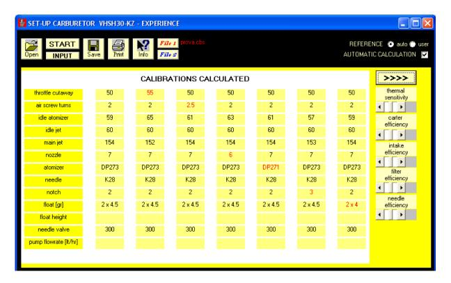
The first calibration calculated maintains fixed all the elements of setting and calculates the jets of the minimum and maximum to be used to optimize it.
