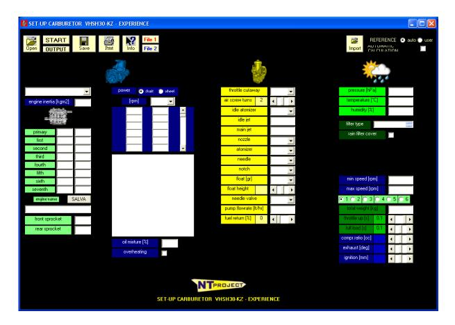
In this new version we have therefore introduced the possibility of inserting the engine power curve. As is known, carburetor calibration is linked to the specific requirements of the engine. With the specific power curve data of the engine it is therefore possible to make a more precise evaluation of the carburetion, and refine the calibration even more in detail.
