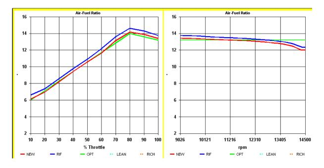
When you modify your starting calibration the red line moves, but the carburation that you had with your starting calibration still remains in the graph in the blue line, so you can see the difference due to your actions.
