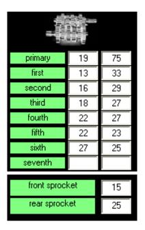
The gear ratios of all the main engines in the category are therefore entered into the software, and it is possible to enter the final ratio used.
