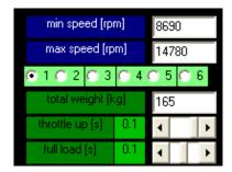
In the calculation of the carburettor calibration, in addition to defining the operating range of the engine where you want to optimize the carburetion, it is possible to evaluate how the carburetion changes in the acceleration phases with the different gears engaged, so will be possible to optimize the setting in the gear shift used in the main corners of each track.
