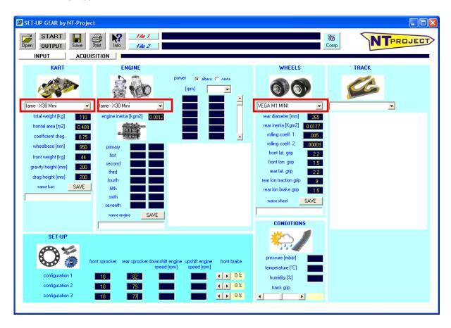
In the SET-UP enter the sprockets of the final drive ratio that you want test, and the brake distribution (if only rear brake click on the right arrow until you read 0%)
